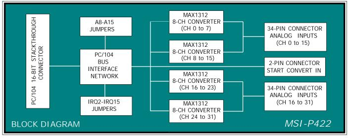
Channels for each of four devices can be enabled or disabled via the configuration register of the devices. Conversion times of approximately 800ns to 2200ns for 1 to 8 channels, respectively, for each device. Since conversions are simultaneous, all four devices are converting at the same time for a maximum time of approximately 2200ns for all 32 channels.
