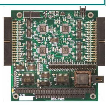
input ranges with capacities of 8, 16, 24 or 32 channels which operate from a single +5V supply with a non-linearity of  $\pm 1/2$  LSB. The inputs are overvoltage tolerant to  $\pm 15V$ . A block diagram of the card is shown in Fig. 1.
